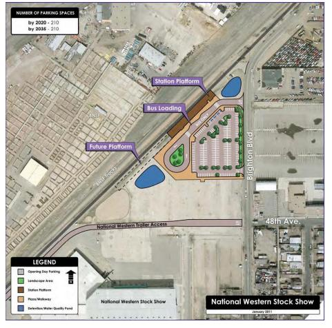
Figure 4-18b: Proposed Station Layout for National Western Complex Station on North Metro Line
